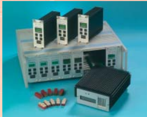
Telemetry system (Transmitter, receiver and power supply)
